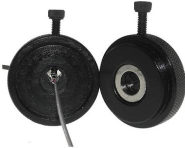
Loosen the screw on the disc that has rotated to access the cable and cut the metal jacket without damaging the cable.
